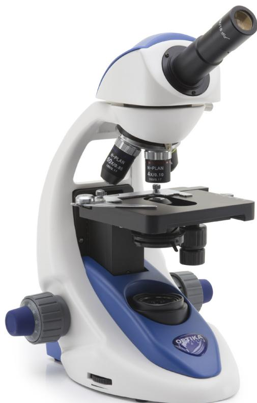
Monocular microscope ideal for teachers and secondary schools, with four N-PLAN objectives (600x), FN 18 high eyepoint, finite optical system, coaxial focusing, mechanical stage, Abbe condenser and powerful, uniform, white color temperature 3 W **X-LED<sup>2</sup>** illumination. Slim and easy to carry, yet sturdy and resistant, it is equipped with all the main controls to start learning how to use an advanced microscope and with long lasting LED illumination to provide over 20 years of use
