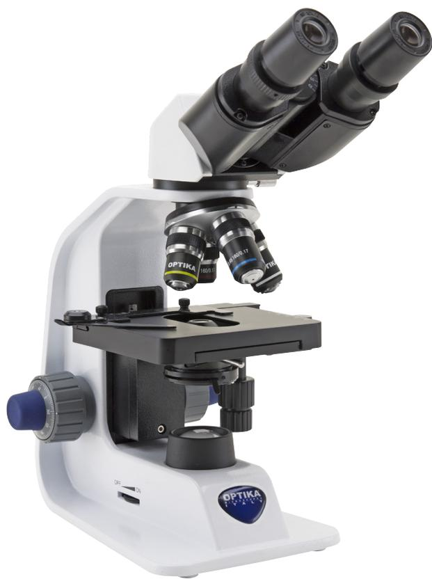
Binocular microscope ideal for students and primary schools, with four achromatic lenses (1000x), FN 18 high eyepoint eyepieces, finite optical system, coaxial focusing, mechanical stage, Abbe condenser and powerful, uniform, white color temperature 1 W **X-LED**<sup>1</sup> illumination. Slim and easy to carry, it is equipped with all the main controls to start learning how to use an advanced microscope and with long lasting LED illumination to provide over 20 years of use
