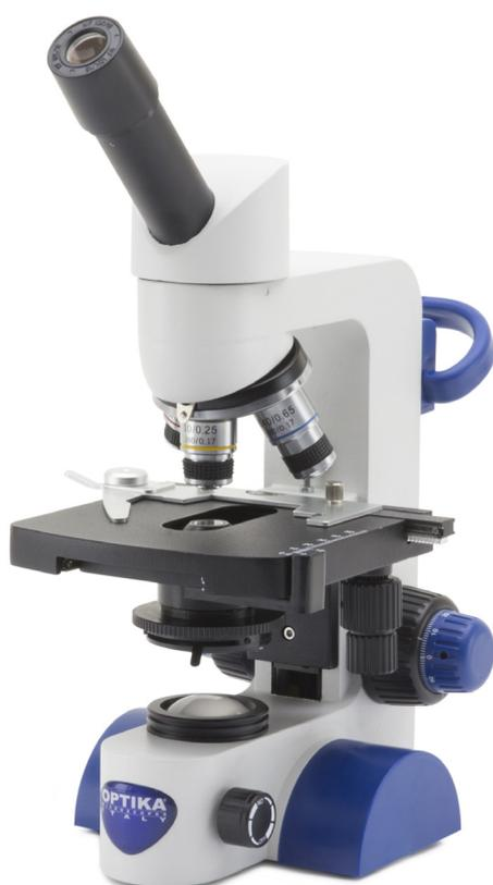
Cordless, modern monocular microscope ideal for students and mainly primary schools with achromatic lenses (400x), FN 18 eyepiece, finite optical system, coaxial focusing, StagErase™ erasable mechanical stage, Abbe condenser and 1 W LED illumination with rechargeable batteries. Slim and easy to carry, it is equipped with arm/wrist rest support to reduce the fatigue during use and long lasting LED illumination to provide over 20 years of use
