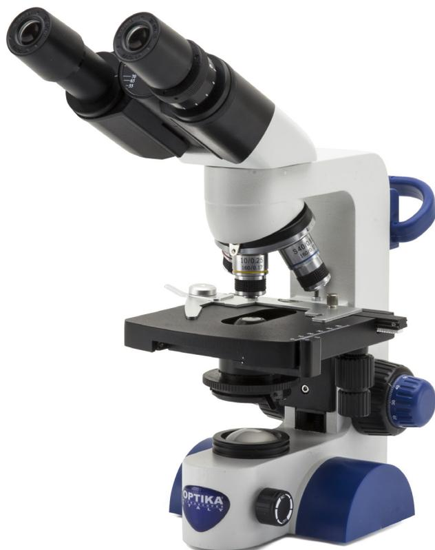
Cordless, modern binocular microscope ideal for students and mainly primary schools with achromatic lenses (400x), FN 18 eyepieces, finite optical system, coaxial focusing, StagErase™ erasable mechanical stage, Abbe condenser and 1 W LED illumination with rechargeable batteries. Slim and easy to carry, it is equipped with arm/wrist rest support to reduce the fatigue during use and long lasting LED illumination to provide over 20 years of use
