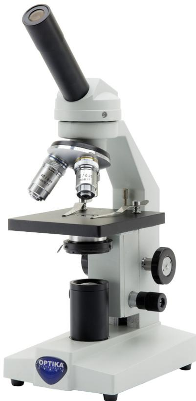
Monocular microscope ideal for students and mainly primary schools, with achromatic lenses (400x), FN 18 eyepiece, finite optical system, coaxial focusing, fixed stage and fixed 1 W LED illumination. Slim and easy to carry, it is equipped with long lasting LED illumination to provide over 20 years of use
