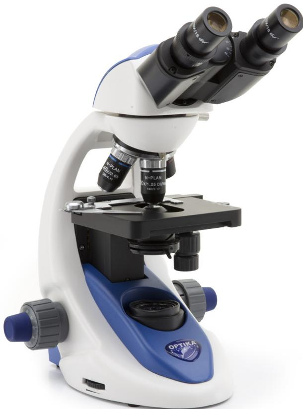
Binocular microscope ideal for teachers and secondary schools, with four N-PLAN objectives (600x), FN 18 high eyepoint, finite optical system, coaxial focusing, mechanical stage, Abbe condenser and powerful, uniform, white color temperature 3 W **X-LED<sup>2</sup>** illumination. Slim and easy to carry, yet sturdy and resistant, it is equipped with all the main controls to start learning how to use an advanced microscope and with long lasting LED illumination to provide over 20 years of use
