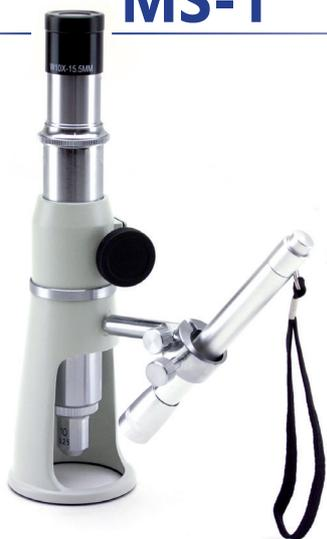
Portable monoscope ideal as multifunctional testing equipment especially for surface analysis and measurements to be used directly on the specimen. Equipped with fixed objective (10x), FN 15.5 eyepiece with crosshair and 0.3 W LED penlight for incident illumination powered by rechargeable batteries
