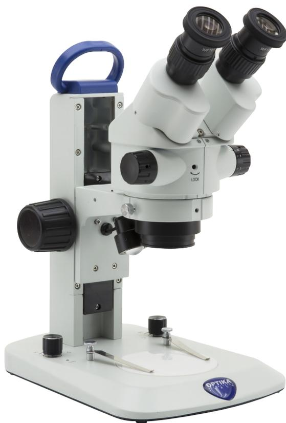
Cordless binocular stereozoom microscope ideal for industrial purposes and students/amateurs to dissect and discover mainly biology and materials science in 3D, with 0.7x...4.5x zoom, FN 21 high eyepoint eyepieces, precision fixed arm with handle and the latest technology of EcoLED™ illumination plus rechargeable batteries. Slim and easy to carry, it is equipped with long lasting LED illumination to provide over 20 years of use
