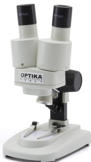
Cordless entry-level binocular stereomicroscope ideal for kids to dissect and discover mainly biology and materials science in 3D, with fixed objective (2x), FN 16 eyepieces, fixed stand and 0.1 W LED incident illumination and rechargeable batteries. Slim and easy to carry
