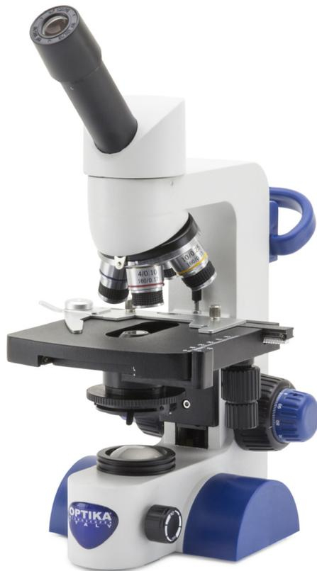
Cordless, modern monocular microscope ideal for students and mainly primary schools with achromatic lenses (600x), FN 18 eyepiece, finite optical system, coaxial focusing, StagErase™ erasable mechanical stage, Abbe condenser and 1 W LED illumination with rechargeable batteries. Slim and easy to carry, it is equipped with arm/wrist rest support to reduce the fatigue during use and long lasting LED illumination to provide over 20 years of use
