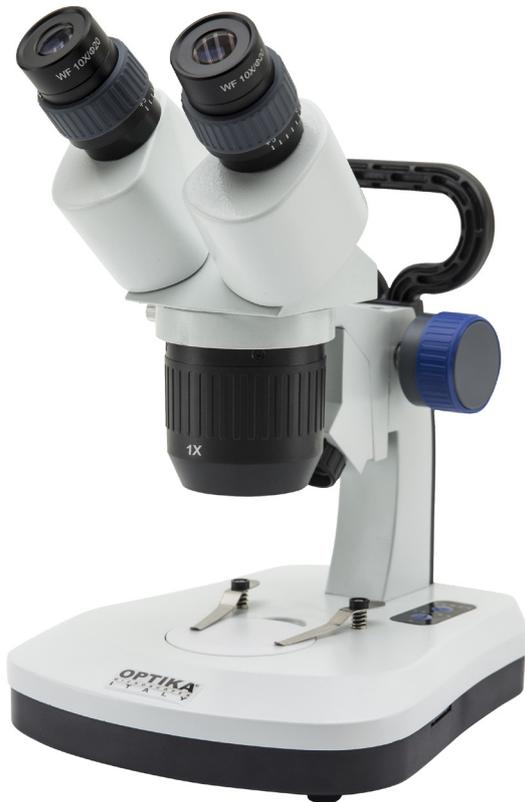
Cordless binocular stereomicroscope ideal for students, schools and amateurs to dissect and discover mainly biology and materials science in 3D, with turnable objective (1x-3x), FN 20 eyepieces, 360° rotating head, fixed arm with handle and 1 W LED transmitted / incident illumination with comfortable touch control and rechargeable batteries. Slim and easy to carry, it is equipped with long lasting LED illumination to provide over 20 years of use
