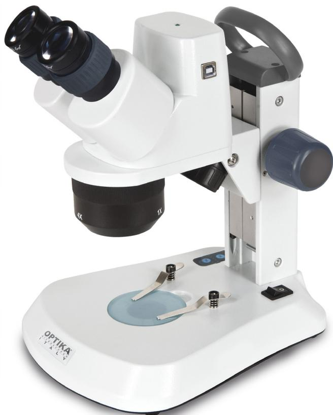
Cordless digital binocular stereomicroscope ideal for students, schools and amateurs to dissect and discover mainly biology and materials science in 3D, with turnable objective (1x-2x-4x), FN 20 eyepieces, precision fixed arm with handle and 1 W LED transmitted / incident illumination with comfortable touch control and rechargeable batteries. Slim and easy to carry, it is equipped with long lasting LED illumination to provide over 20 years of use
